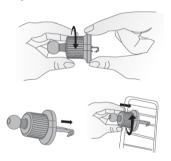
Place the hook and latch it on to your air vent. Screw the adjustment anti clockwise to tighten the adjustment and fix the mount securely to your air vent.
