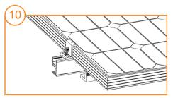
Install two end clamps to secure the panel on the left side by tilting rail nuts into rails, then fasten the two M8\*25 inner hex bolts of end clamps.
