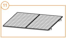
Secure the panel on the right side of an array by two end clamps installed in the same way.
