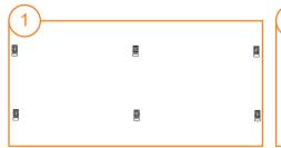
Install all the needed L feet onto the roof.
