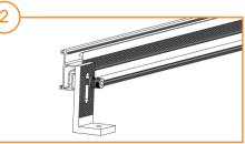
Install a M8\*25 inner hex bolt and a rail nut loosely onto the L foot, then tilt the nut into the rail groove. Fasten the bolt to secure the rail.
