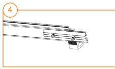
Put half of a rail splice kit into one end of the rail.
