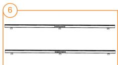
Install all the rails to L feet and use rail splice kit to connect two rails.
