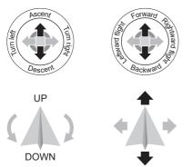
Mode 1 operation: Left joystick controls forward, backward, turning left/right. Right joystick controls flight height, left/right side flying.
