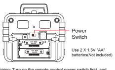
Pairing: Turn on the remote control power switch first, and then turn on the car power switch. When the remote control light changes from flashing to constant lighting, pairing is completed. Trim Adjustment: Adjust the jog lever on the bottom of the car so that the car can drive along a straight line.
