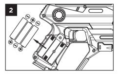
Insert 3 AAA batteries(not included). Make sure the batteries are inserted with the correct polarity.
