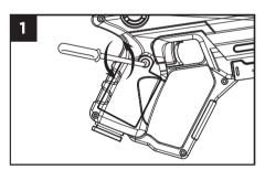
Use a screwdriver to remove the battery cover
