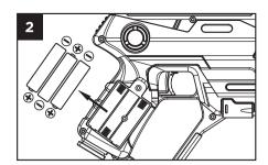
Use a screwdriver to remove the battery cover
