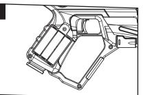
Insert 3 AAA batteries(not included). Make sure the batteries are inserted with the correct polarity.
