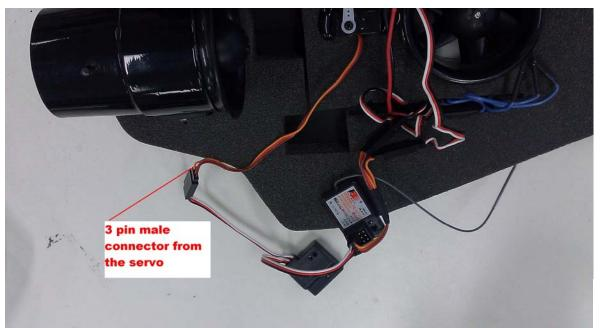
Step 4: Mount the gyroscope module into the provided space using the attached double sided tape, and neaten up wires
