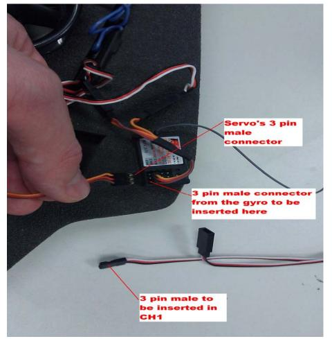
Step 2: Plug the gyroscopes male 3-pin connector from the gyro into Ch.1 on the receiver
