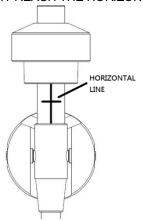
FOR OTHER CARTRIDGE, USER CAN ADJUST THE TRACKING FORCE BY TURNING COUNTERWEIGHT INWARDS OR BACKWARDS. TURN THE CUONTERWEIGHT INWARD TILL IT REACH THE HORIZONTAL LINE. HOLD THE COUNTER WEIGHT WITH ONE HAND, TURN SCALE RING TO "0" AGAINST THE INDEX LINE ON THE SHAFT WITH ANOTHER HAND, BE SURE NOT TO TURN TOGETHER WITH THE
