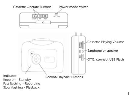
**NOTE:** Please press the cassette PLAY button after the deck door close completely, otherwise may cause the movement damage.
