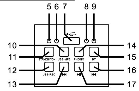
5 STANDYBY/ON indicator7 USB socket9 BT indicator11STANDBY/ON button
