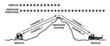
Your XRS-330C radio allows you to enable or disable Duplex mode on individual repeater channels. In this way any repeater channels that are not being used with repeaters in your area can be used in Simplex mode for normal direct radio-to-radio communications.
