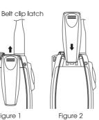
2.3 Installing the supplied NI-MH Rechargeable Battery Cover (Battery built-in to the battery cover)
