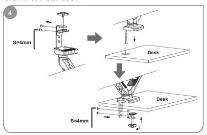
Loosen the two screws on the base, pass it through the hole in the table, and screw in the two screws that have just loosened
