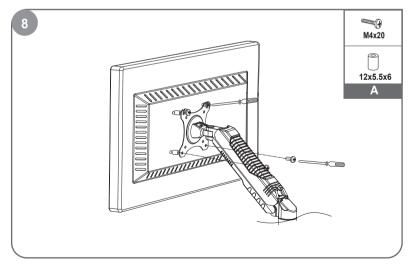
Recessed surface installation:Put spacers between headplate and monitor. Install the lower two screws and fasten the upper two screws.
