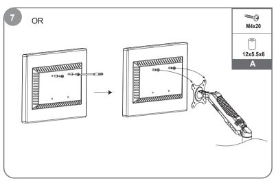
Recessed surface installation:Put spacers between headplate and monitor. Install the upper two screws and don't screw them tight. Leave some space and hang the monitor on the head plate.
