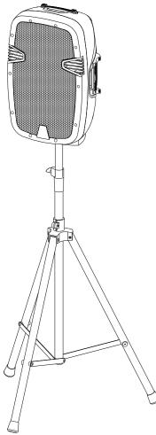
**Pole Mounting**: This series also include a pole mount option. The pole mount socket located on the bottom of the speaker may be used to secure the speaker to a speaker tripod. Always be sure to fellow the guidelines listed be blow when pole mounting your speaker.
