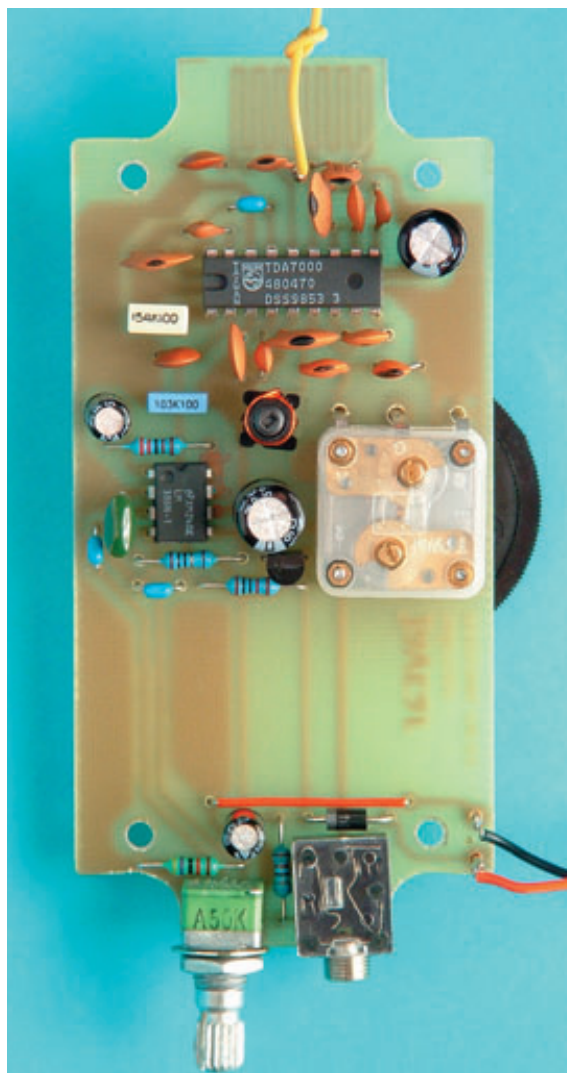
Here's the circuit diagram (top), the wiring diagram (above) and the closeup top photo of the FM Radio's PC board assembly (left). Use them all as a guide when you're building up your own Radio.
