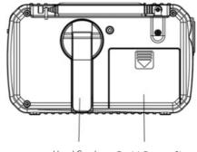
Hand Crank 3 x AA Battery Slot
