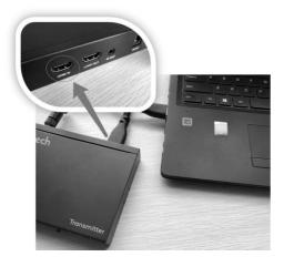
Connect the Transmitter to your media output device through the "HDMI IN" port.
