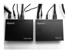
**03** Connect the Receiver and Transmitter with the 3.5mm male to male cable.
