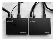
Connect power to Transmitter and Receiver separately.
