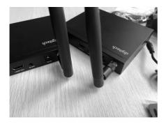
Install antennas for Transmitter & Receiver.
