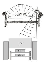
2) The front of the receiver should directly face the audio/video remote sensor.
