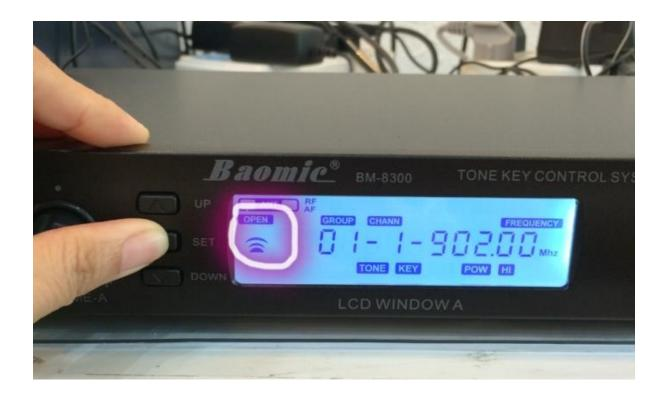
5. Open the front cover of the spare microphone and face it towards the IR transmitter of the receiver until the screen indicates they are paired..
