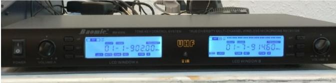
2. Push the "SET" button for 3 secs to unlock the receiver.
