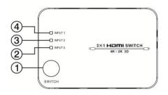
**Front Panel:** Connect the output of the switcher to a monitor or HDTV that is equipped with a HDMI socket. The selected source will be displayed from this output.
