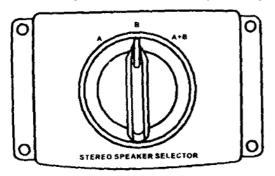
**Caution:** This speaker selector switch is limited to a maximum of 10 watts/channel, continuous music power.
