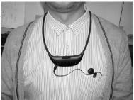
(2.6) When you go out, take the receiver and your hearing aid. Put the microphone cable in your pocket, clip on the jacket. It can be worn as a normal hearing aid.
