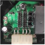
ON 1 Min LK4 is set; LK3 is set to M; LK1 is set to 1: OFF 1 Min LK6 is set; LK5 is set to M; LK2 is set to 1.
