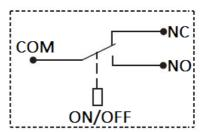
When power is applied, the relay will switch the connection from the Normally Closed NC position, to the Normally Open NO (ie: now closed).
